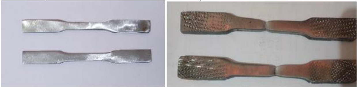
Figure 5. Simple tensile test specimens before the test (LHS) and after the test (RHS).
