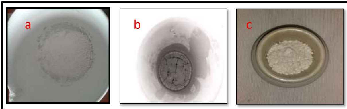
Fig. 2. Materials used (a) TiO 2 Nps, (b) CTRD, (c) CTPD, after calcination at 300 °C for 2 hours.
